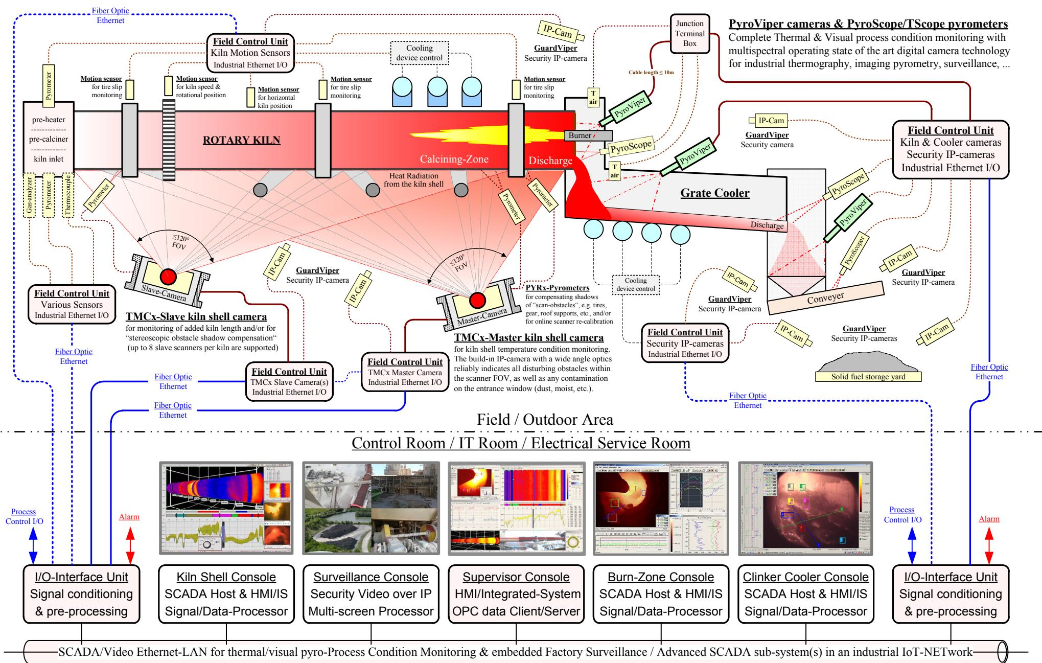
Data-link to the Field-, Control-, or Operations- Level of a Plant Automation System via industrial Ethernet communication
